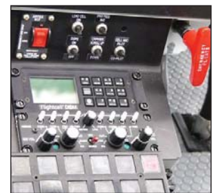
Below: Installed view of the Flightcell DZM
