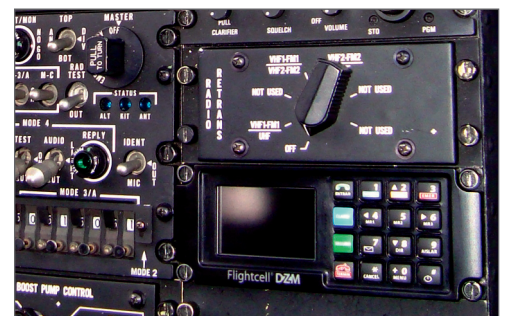
Left: Flightcell's Iridium 9505A Phone Mount. Below: Installed view of the Flightcell DZM2 (H60 Blackhawk)
